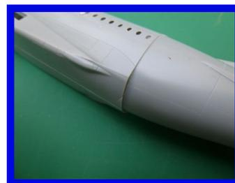
13. Sand the end of the tailcone to accept a piece of 3/16" rod (or sprue) and shape and drill to represent the APU. Add the windscreen and blend in. Mask the wing, engines, tail and fin mounting surfaces to keep paint off them. Give the fuselage an overall rub with a 12,000 grade polishing pad to prepare it for painting.
