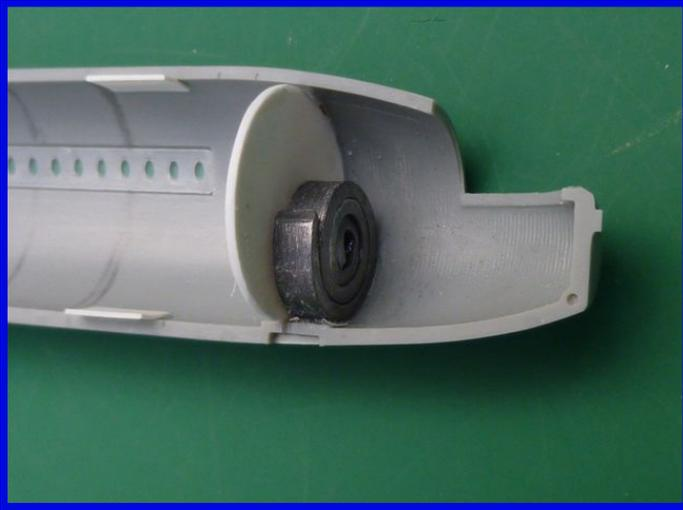
5. Fit the clear windows to both fuselage halves and make flush since the windows will be represented by decals from the STS decal sheet. Some of the clear windows are proud whilst others are undercut and will need filling and sanding flush. Note that the plastic surrounding the window inserts is half the thickness of the fuselage moulding and excess cement will dissolve it.
