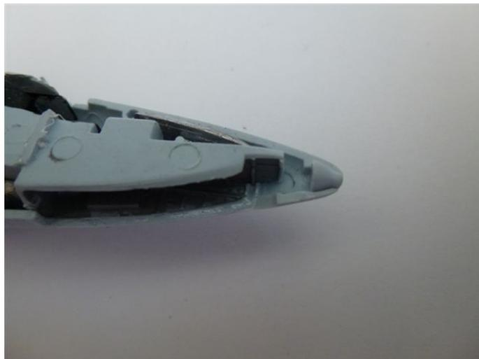
7. 2gm of nose weight is recommended, but this will not fit above the nose wheel bay. Strip lead will fit under the tub and behind the rear bulkhead and 3gm balances the model (see photos 1 to 3)
