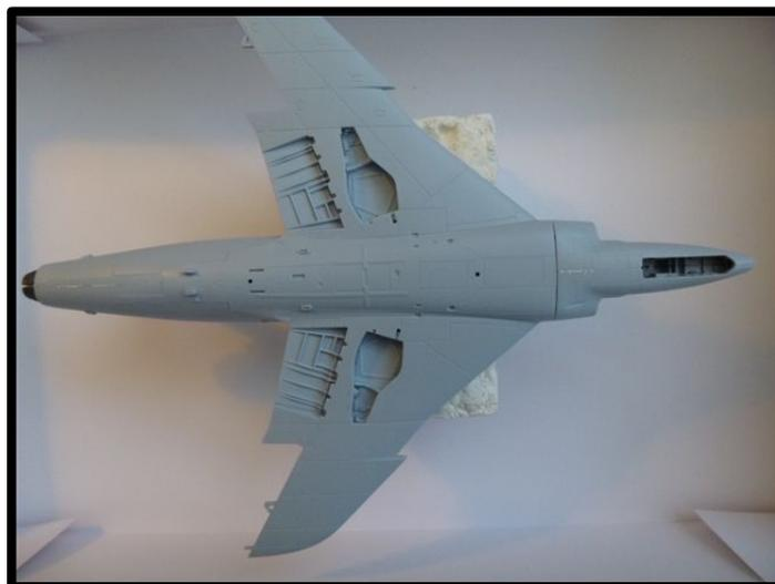
10. Step 21 - fit the rudder and ailerons (Steps 24/25) but don't fit the tailplanes, flaps, landing gear, doors and pitot head until you have finished masking, painting and decaling.
