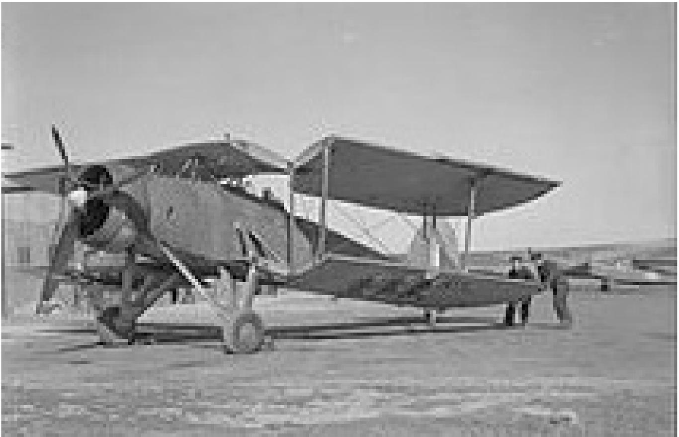
2391 were built...the Fairey Company's most famous aircraft all fitted with a Bristol Pegasus radial engine of 690 hp which was later upgraded.
